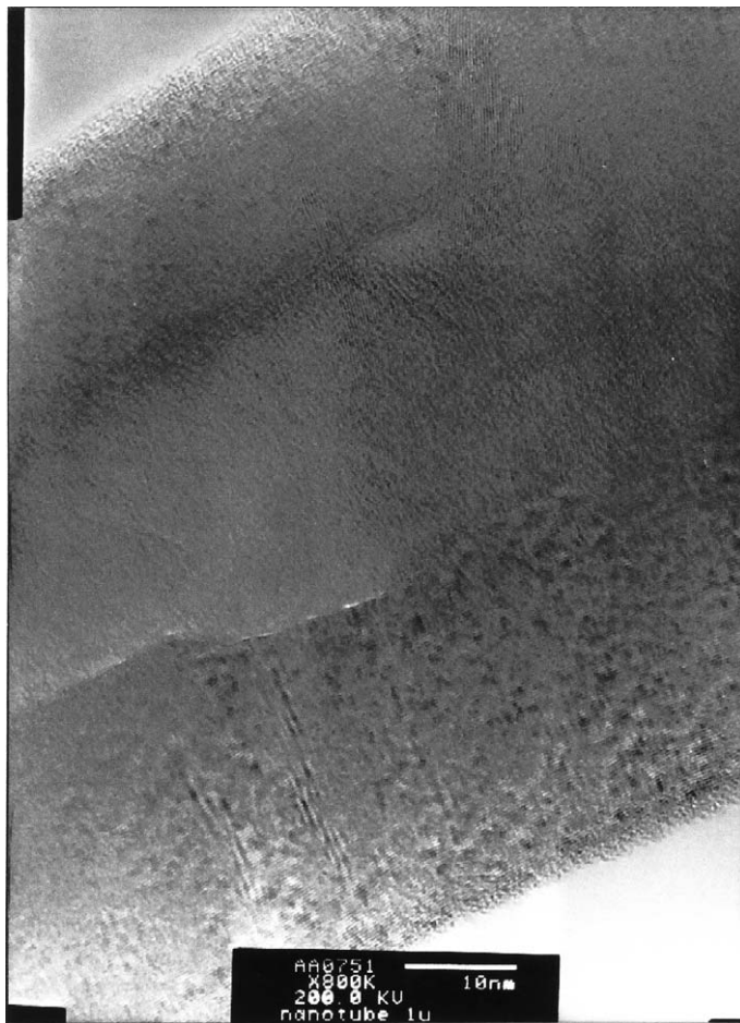
Fig. 1. C-MWNT magnified 800,000 times.
